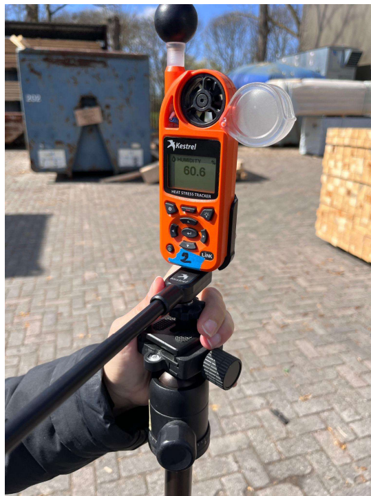
Figure 6 Ground-level view of the Kestrel 5400 Heat Stress Tracker 2 (Terminal), positioned on paved terrain surrounded by industrial containers and equipment ( 51^{\circ} 53' 15.58'' N, 4^{\circ} 23' 50.67'' E).
